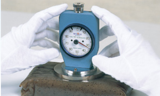
Hardness measurement of Konjac. Durometer : GS-744G
