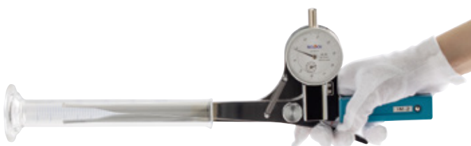
The bore diameter of deep part is 23.1mm. Inner Caliper Gauge : IM-2
