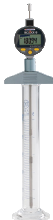
The inner depth is 180.94mm. The length of stylus is extended by the extension rods. Depth Gauge : SSD-215
