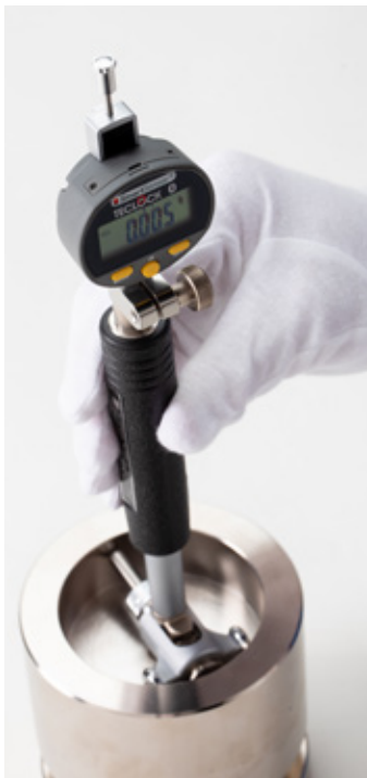
Comparative measurement of inside diameter by Bore Gauge
