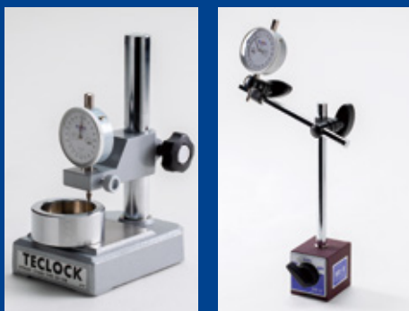
Mounting a dial indicator on a stand or a magnet base stand.
