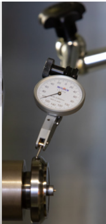
Comparative measurement by Test Indicator
