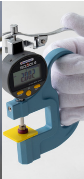
Direct measurement by Thickness Gauge
