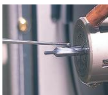
The photo shows the scene of detecting deflection of cutting tool edge installed to the machine and deflection.
