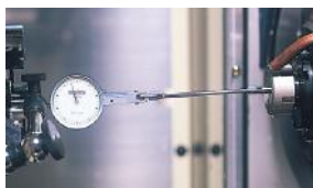
The photo shows the scene of detecting deflection of cutting tool edge installed to the machine and deflection.
