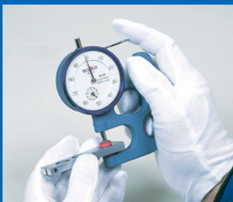
Measuring metal work piece. The photo shows 5.98mm.
