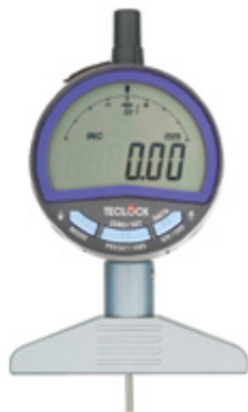
DMD-211A φ2 Flat Needle Contact Point
