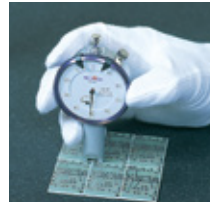
V-Grooved depth measurement of Print circuit board by using DM-251.
