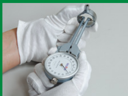
Measuring example of inner diameter of a small metal work piece.
