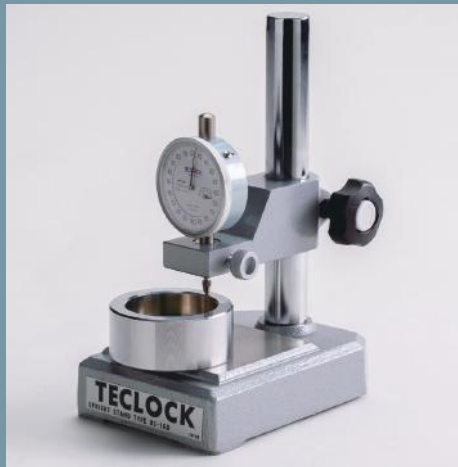
It is measured a work piece by mounting dial indicator on a stand.
